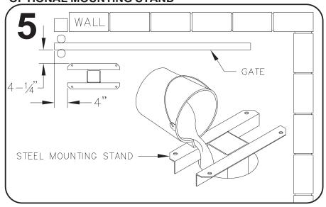
O If the steel mounting stand will be used, place the shortest edge of the stand 4" from the driveway edge and place the longest edge of the stand 4-1/2" away from the gate. The top of the steel stand may sit on the ground or the stand may be elevated to keep the operator above snow, flooding etc. Make a post hole and cement the stand in place, making sure the stand is level and square to the gate.
